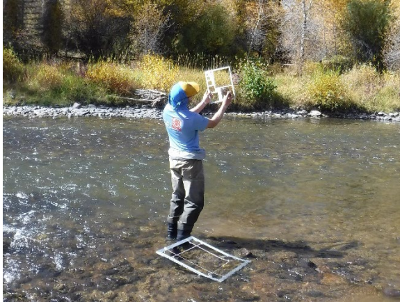
Photo 3-1: Substrate being measured with a gravelometer at Site CR-16.7 on the Colorado River.
