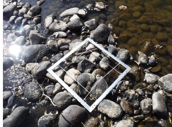
Photo 3-2: Sampling frame with four cross sections for randomized substrate characterization.
