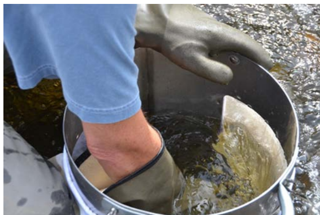
Figure 6 - Sample Collection with a Hess Sampler
