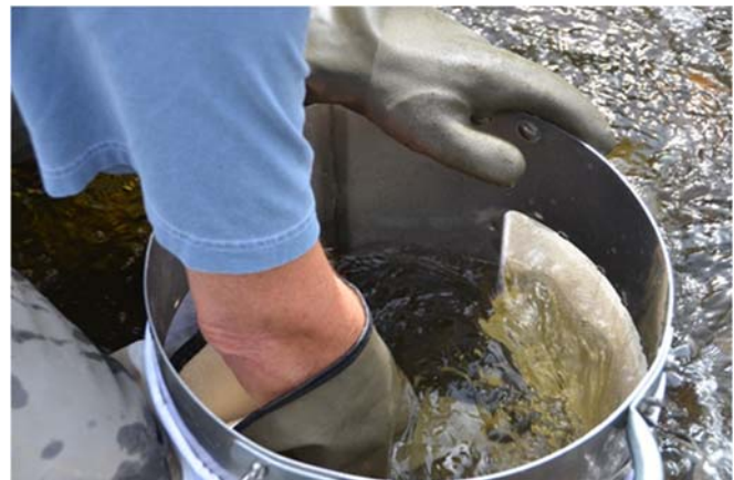
Sample Collection with a Hess Sampler
